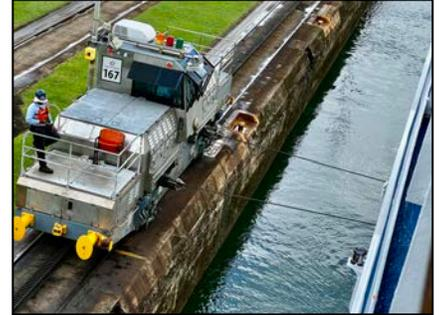
One of the four engines that pulled the ship through the Panama Canal
